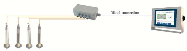
CONNECTION IN SERIAL (FROM 4 up to 8 Load Cells)
